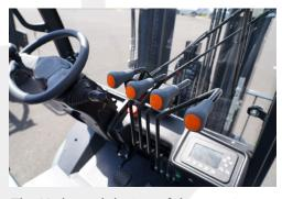
The U-shaped design of the steering wheel and the front-mounted multi-directional valve control make driving easy.
