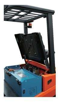
The standard design of the fully accessible bonnet makes daily maintenance practical and efficient. The battery can be replaced very quickly, allowing continuous operation.
