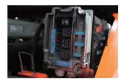
The main electronic components are protected and housed in a special casing for enhanced protection (temperature, vibrations, dust, water splashes, etc.).
