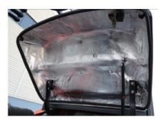
The engine is housed in an enclosure designed to prevent the ingress of dust, water and other contaminants.
